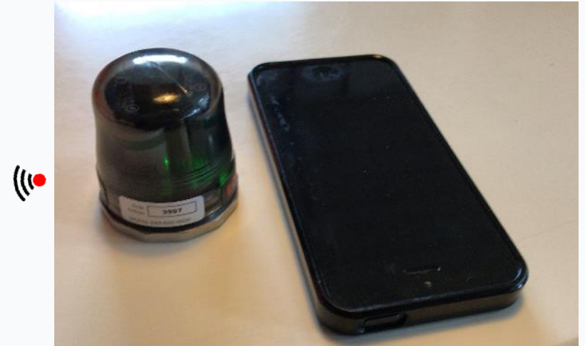
Ventus RCM wireless and battery powered sensor node located next to iphone5
